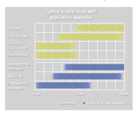
Mesh pads are often used in evaporators and separation columns to prevent liquid from getting carried into the gas flow. They are also utilised in cooling systems condensers and after scrubbers to protect the system from liquid spray.
