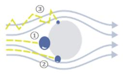
Special fibers are the heart of our fiberbed mist eliminators. Fabricated with highest precision and supported by a solid cage the special fibers are able to reliably remove even submicron particles. Droplets bigger than  $1\mu$ m are removed by impact ① or interception ②.
