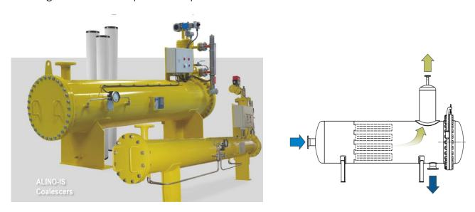
After the oil-water mixture has flowed through the coalescence elements, two phases are formed. Oils or other hydrocarbons rise and collect in a separation chamber.
